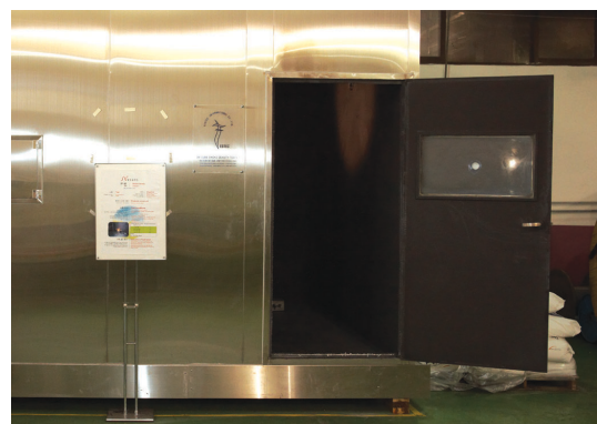
27 m 3 cube smoke chamber
